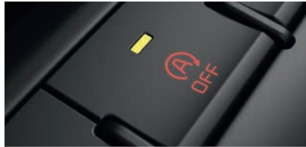
**Idle Stop & Go (ISG).** ISG comes as standard on all Picanto models and is designed to reduce fuel consumption by shutting down the engine when the vehicle is at a standstill.
