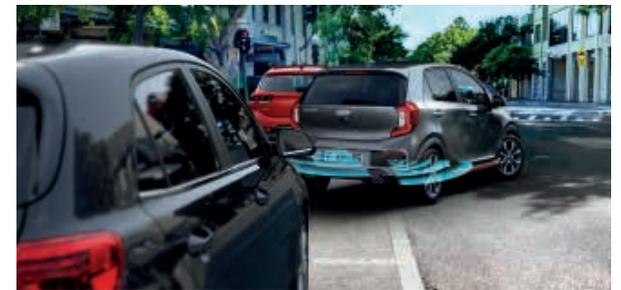
**Rear parking sensors.** Ideal for confident parking, these ultrasonic sensors mounted on the rear bumper warn you of any obstacles when manoeuvring into a parking space.
