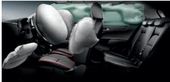
**Front/side/curtain.** To help protect occupants and potentially reduce injuries in the event of a collision, the Picanto offers driver and front passenger airbags, two front-side airbags and two side-curtain airbags.
