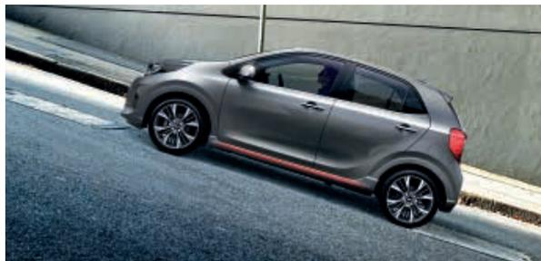
**Hill-start Assist Control.** When at a standstill on an incline, Hill-start Assist Control prevents you from rolling backwards. It applies the brakes from the time you lift your foot from the brake pedal, giving you a moment to switch your foot smoothly to the accelerator.
