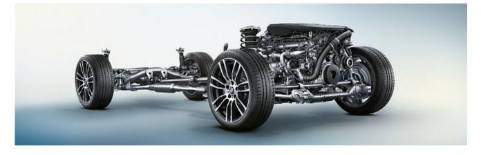
An ideal **axle load distribution** of 50:50 helps ensure great directional stability, agile handling and a precise steering response. A lower centre of gravity, along with a long wheelbase with short overhangs, generates optimal conditions for these positive driving characteristics.
