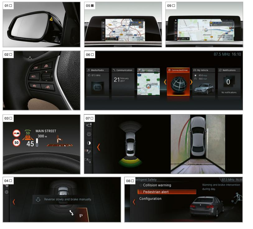
**[01]** Lane Change Warning alerts the driver during lane changes if there is a vehicle in the driver's blind spot or approaching on the adjacent lane by using a visual signal and vibrating the steering wheel.
