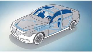
Airbags for the driver and front passenger along with head and side airbags provide strategic protection. The rigid passenger cell provides the best possible passive safety in the event of a front, side or rear collision.
