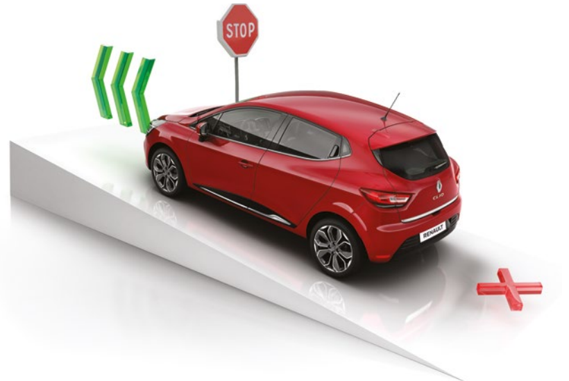
Hill Start Assist (HSA) When starting the vehicle on a hill, the brake pressure is automatically maintained for two seconds, giving the driver time to manoeuvre.
