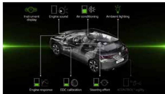
In **Eco Mode**\*, you can make use of the energy-saving eco mode which reduces the steering wheel effort, the engine response, the EDC calibration and the air conditioning capacity.
