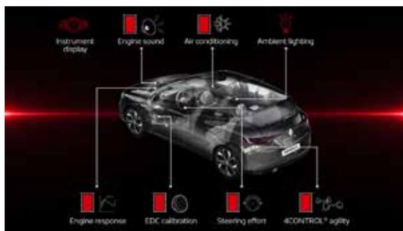
In **Sport Mode**, you use all the features at their full capacity for a sportiest driving experience. The acceleration of the vehicle is quicker, the EDC gear-box ratios are reduced and the 4CONTROL system\*\* generates a sensational sporting responsiveness for increased agility or stability. The steering gets heavier for more precise control.
