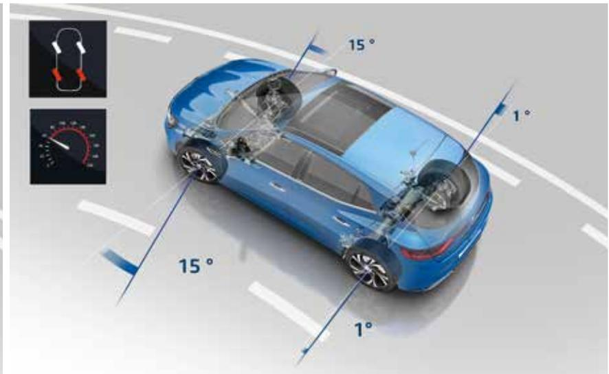
Above 37 mph\*, the rear wheels turn in the same direction as the front wheels.
