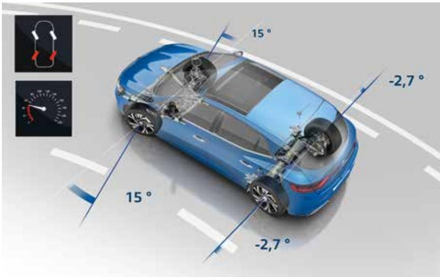
At low speeds, the 4CONTROL system turns the rear wheels in the opposite direction to the front wheels.
